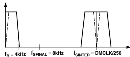
d. Final Filter LPF (HPF) Transfer Function
