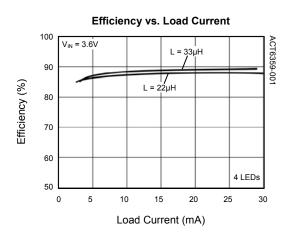
Efficiency vs. Load Current
