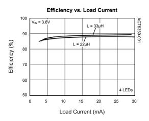
Efficiency vs. Load Current
