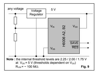
**Version A3, B3:** for monitoring of regulated voltage, where no unregulated voltage is available (the tolerance is  $\pm 10$  %, see Table 4. For tighter tolerances, trimming can be used, see Fig. 10).
