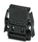
IDC female connector, Nominal current at 20 °C: 1.2 A, Test voltage: 500 V AC, number of positions: 32, pitch: 1.27 mm, color: black, contact surface: Gold
