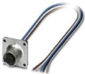
Sensor/actuator flush-type socket, 5-pos., M12, B-coded, front/square flange mounting, with 0.5 m TPE litz wire, 5 x 0.34 mm 2
