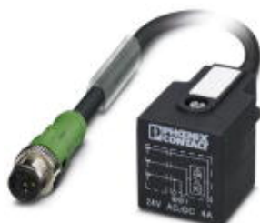
Sensor/Actuator cable, 3-position, PUR halogen-free, Black-gray RAL 7021, Plug straight M12-SPEEDCON, A-coded, on A valve plug, with 1 LED, connected with Z diode, Cable length: 0.6 m
