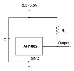
Note: 4. C is for power stabilization and to strengthen the noise immunity, the recommended capacitance is 10nF~100nF.
