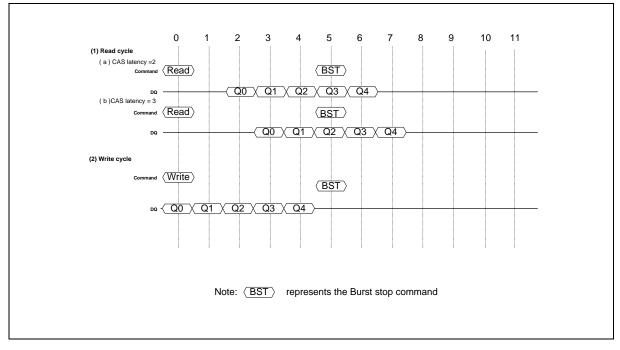
Timing Chart of Burst Stop Cycle (Precharge Command)
