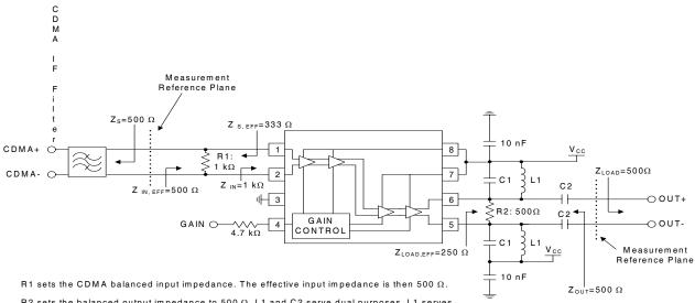
R2 sets the balanced output impedance to 500  $\Omega$ . L1 and C2 serve dual purposes. L1 serves as an output bias choke, and C2 serves as a series DC block. In addition, the values of L1 and C2 may be chosen to form an impedance matching network of the load impedance is not 500  $\Omega$ . Otherwise, the values of L1 and C1 are chosen to form a parallel-resonant tank circuit at the IF when the load impedance is 500  $\Omega$ .
