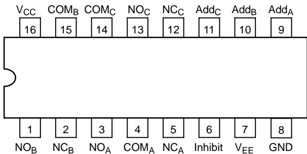
Figure 1. Pin Connection (Top View)
